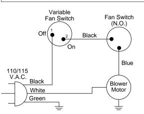
Figure 54 - Blower Wiring Diagram for Thermostat-Controlled Models
